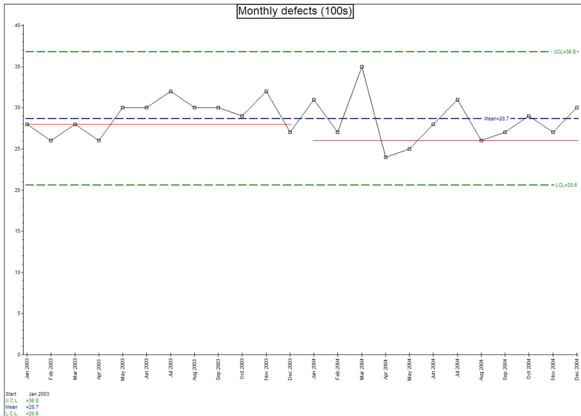
Figure 4 - A Process Behaviour Chart of the monthly defect data
