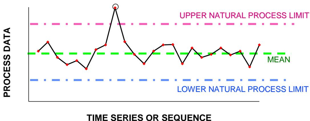
**Figure 3 - A simple diagram of a Process Behaviour Chart**
